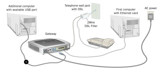
Figure 5. Gateway Connected to Second Computer Via USB
